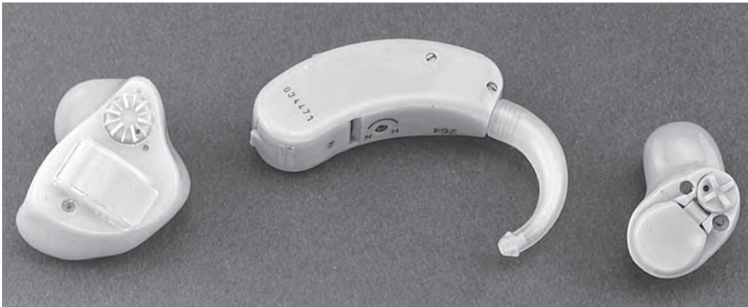
Figure 13.7 Types of hearing aids. Left , in-the-ear; center , behind the ear; right , in-the-canal.
