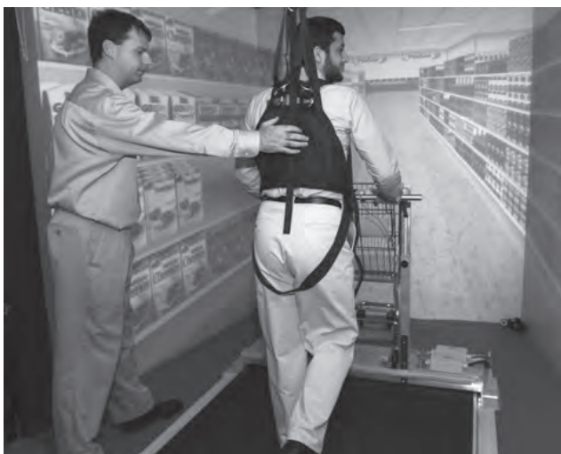
Figure 28.4 The Balance Near Automatic Virtual Environment (BNAVE) was developed in collaboration by the University of Pittsburgh and Georgia Tech. A virtual grocery store is one of the environments developed for the BNAVE. Navigation through the store can be achieved using a joystick (subject is stationary) or pushing on a force-sensitive grocery cart while walking on a treadmill (subject is moving).
